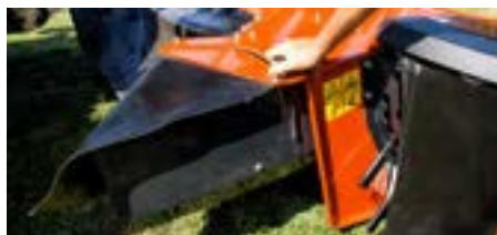
Integrated swath plates, easily adjusted to correct swath width.
