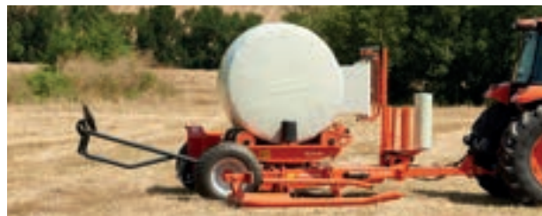
The adjustable loading arm with rear end stopper and inner support tube, allows the bale to be picked up and loaded on the move.
