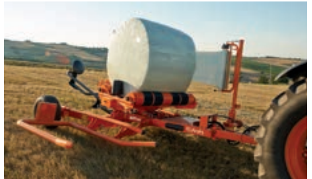
Turntable with two driven rollers designed for a high bale stability and smooth even rotation.
