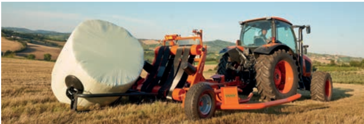
The Kubota Turntable wrappers can be fitted with a bale turner as an option.
