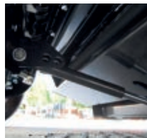
Standard fit hydraulic pick-up lift for reduced downtime between jobs and added in field convenience.
