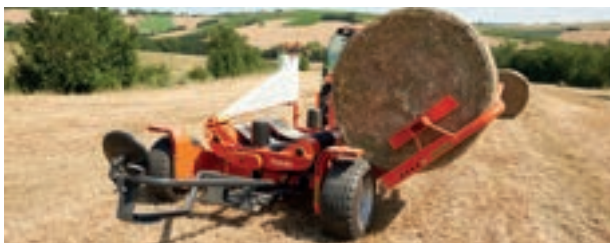
The short lifting height provides fast transfer of bale from arm to turntable.
