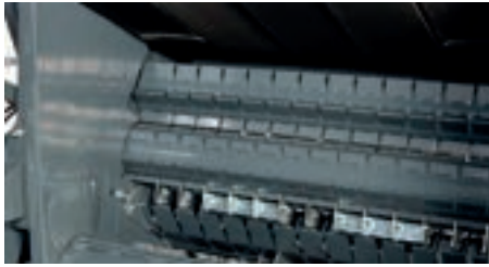
The two front rollers with self-cleaning scrapers are designed to work well in silage and provide instant bale formation.
