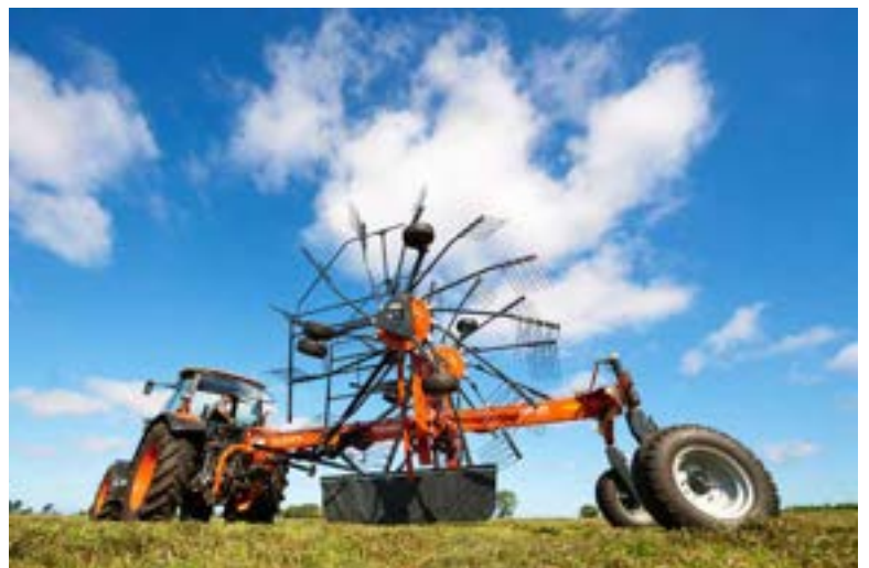
Kubota RA2584 is converted hydraulically for transport position from tractor cab.
