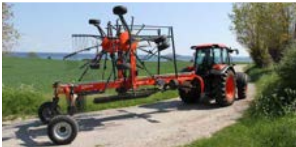
To limit transport height further the tine arms can be removed on the RA2076. The swath board folds up automatically.
