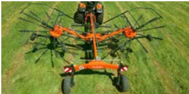
The hydraulic adjustable rotors on RA2076 can be set between 22'9" (7.00m)...
