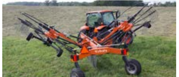
The ability to make sharp turns up to 80° and the cross stabilizer in the headstock are Kubota features.
