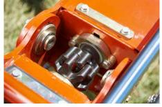
Kubota HexaLink finger clutch permits a 180° folding of the rotors for transport.
