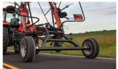
The wide track of the transport wheels ensures stability during roading of the machine.
