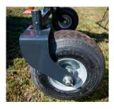
Optional third wheel with tandem axle for high accuracy in ground followings.
