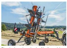
Standard running wheels of both models are extra wide 10.0/75 – 15.3 tyres with a generous track width of 8' (2.45m).
