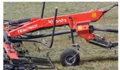
A third wheel allows for better tracking and more accurate tedding action. This wheel also helps adjust the tedding height.
