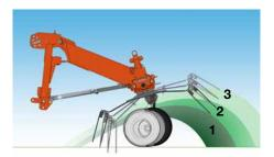
Easy adjustment of spreading angle via pin holes, no tools required.
