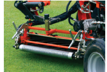
Unique swing out center cutting unit for ease of service
